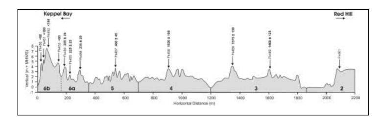
Figure 3: A surveyed cross-section of the beach ridge plain at Long Beach, on the western margin of Keppel Bay. Five accretion units (sets of ridges) are indicated by numbers (6b - 2).
